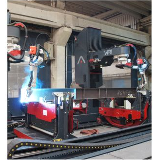
ROBOTIC STRUCTURAL STEEL BEAM ASSEMBLY AND WELDING
