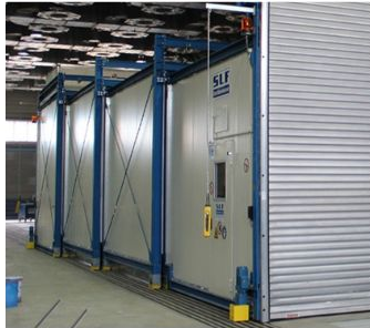
PAINT DRYER SYSTEMS
