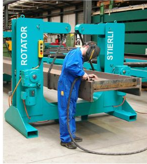
BEAM WELDING / ROTATION
