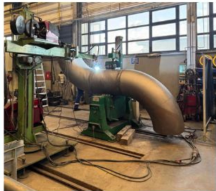
PIPE ROTATORS AND PIPE WELDING
